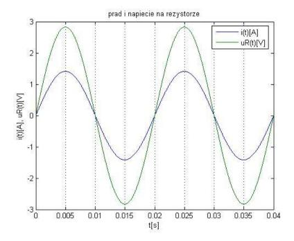
Picture 1. Current and voltage waveform of resistor R.
