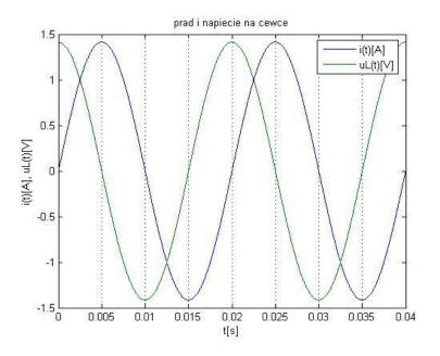
Picture 2. Current and voltage waveform of inductivity L.
