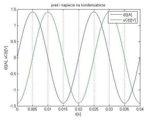
Picture 3. Current and voltage waveform of capacitor C.
