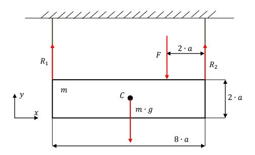
As is seen from drawing, forces work only in y axis direction.
